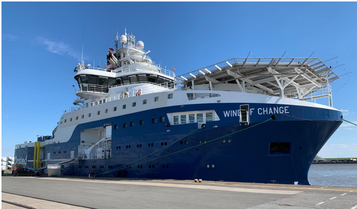
Figure 57: Service Operation Vessel (SOV) - Wind of Change owned by Orsted
