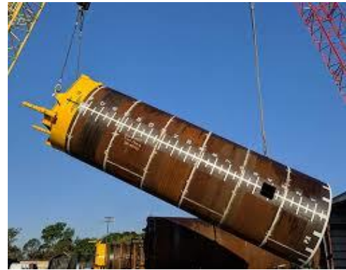
Figure 87 - Suction Anchor from Acteon
