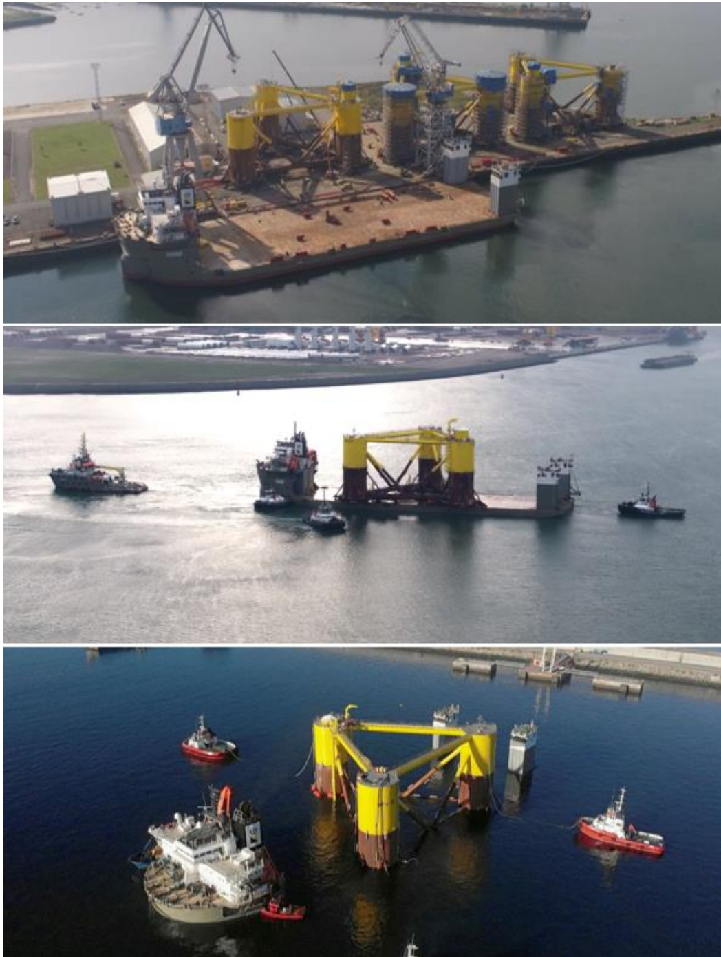
Figure 59: Platform loadout – Roll-on-roll-off
