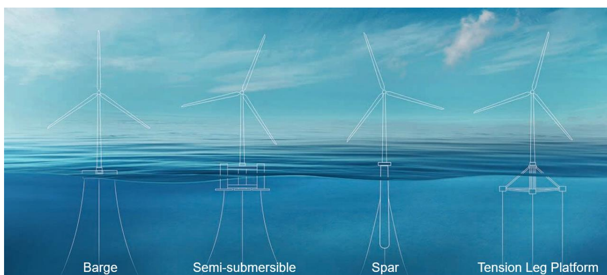
Figure 78: FOW Foundation Types [Image Credit : DNV GL]
