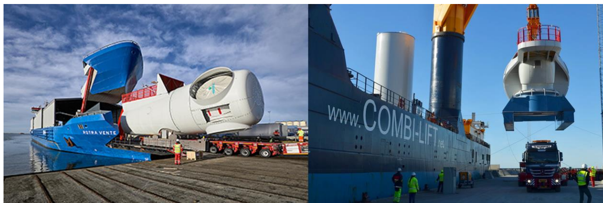
Figure 56: Nacelle offload options (Ro/Ro or Lo/Lo)
